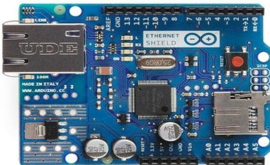
Gambar 2. Ethernet Shield
