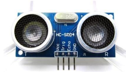
Gambar 3. Sensor ultrasonik HC SR04
