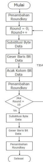
Gambar 10: Flowchart Proses Enkripsi AES-128
