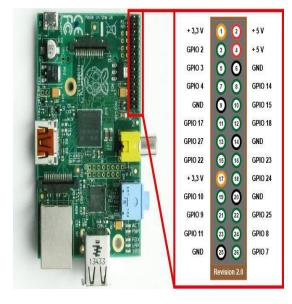
Gambar 3. Skema GPIO Raspberry Pi
