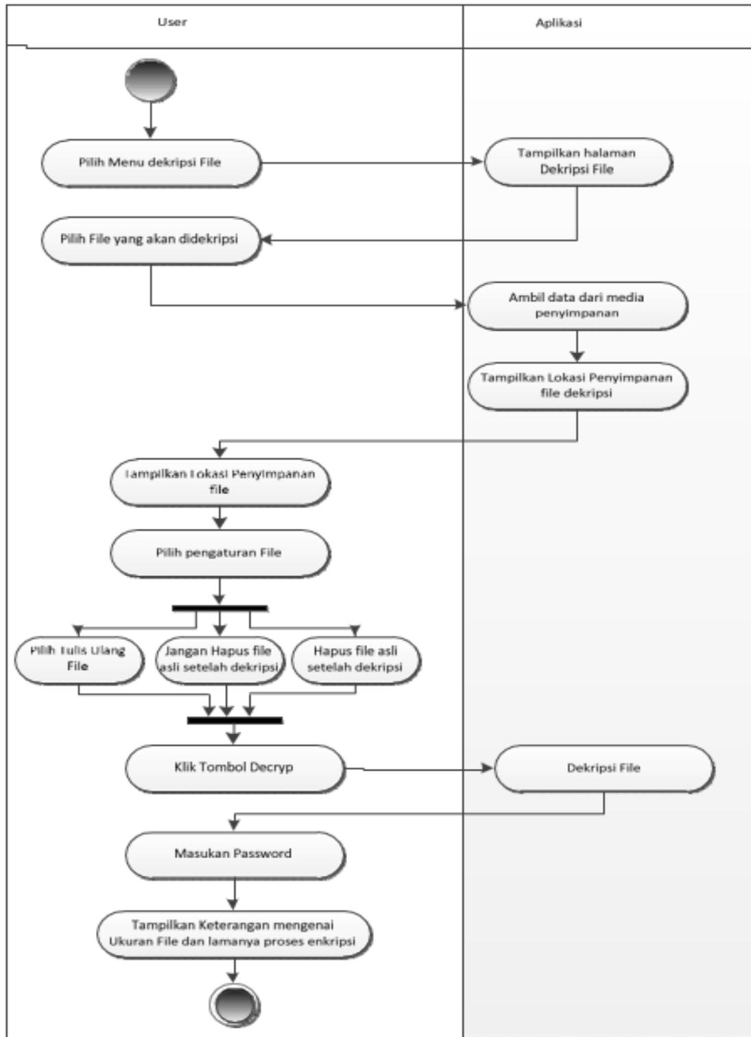
Gambar 5. Activity Diagram Proses Dekripsi
