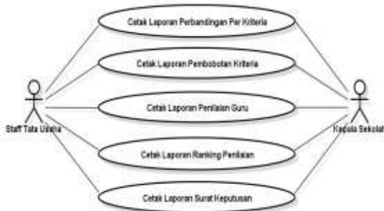
Gambar 4. Use Case Diagram Proses
